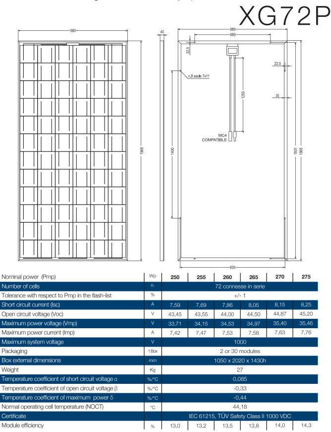
All data at standard testing conditions: STC = 1000 W/sq.m.,AM 1,5 25°C
